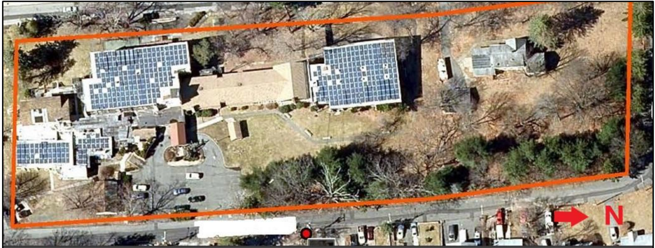
Photo 3. An aerial photograph of the assisted living facility. The red dot at the bottom of the picture indicates the closest fire hydrant. (Photo courtesy of the county Fire Academy)
